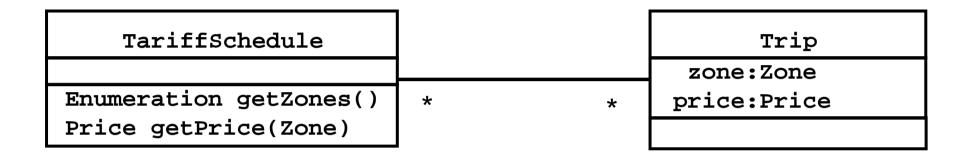
Class diagrams represent the structure of the system.
